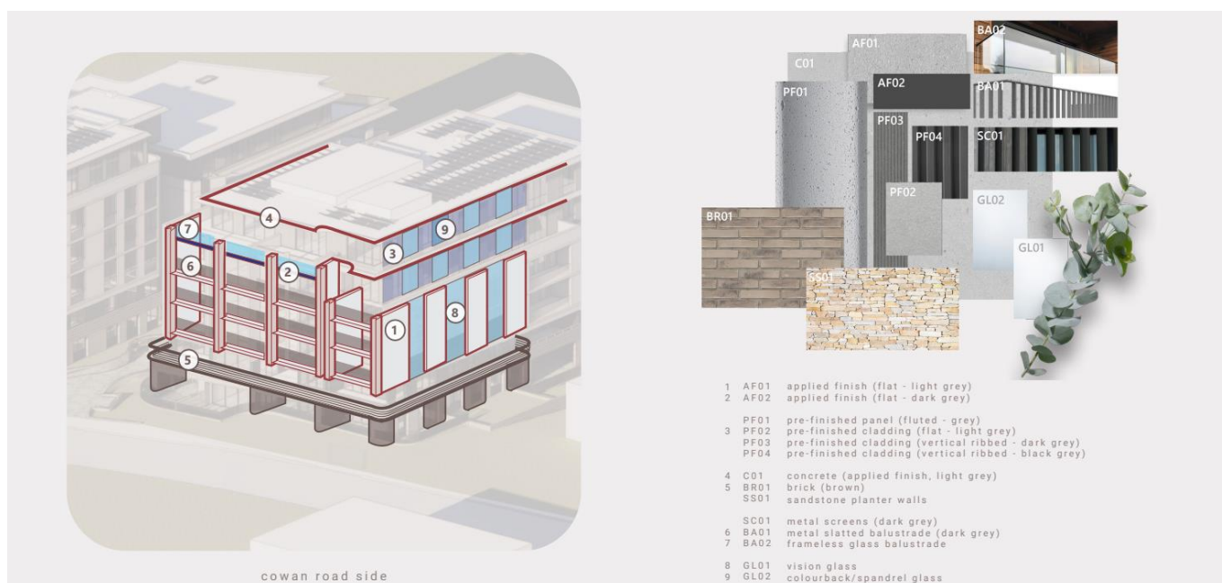
Figure 14 Facade concept Cowan Road side
